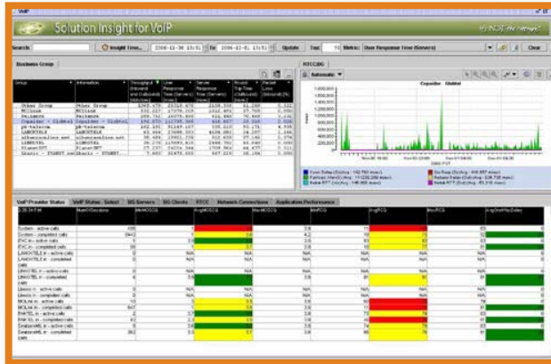
The NetSensory Solution Insight for VoIP lets you track the MOS ratings or other metrics for calls aggregated by Business Group (e.g., remote office) and service provider, yielding a real-time and historical view of service level delivery.
